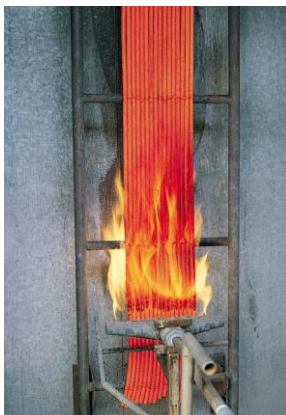
FR-LSZH Cable being tested for Tray Cable Flame IEEE-383
