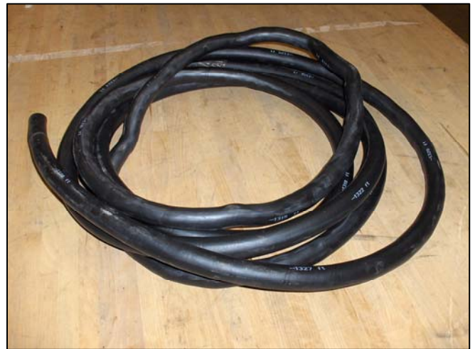
Brand F – Foreign Cable after Flex Test Note: Severe twisting after only 450 cycles
