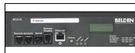
Intelligent PDU Communication and Environmental Monitoring Ports
