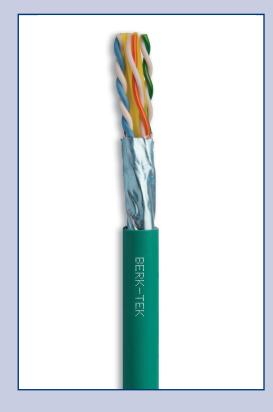
The LANmark-XTP cable features an innovative noise cancelling tape that provides a 4 dB improvement in alien crosstalk performance margins when compared to a standard CAT 6A UTP cable. This improvement in alien crosstalk performance provides a reduction in frame error rates, fewer retransmissions, improved noise immunity and a more reliable network.
